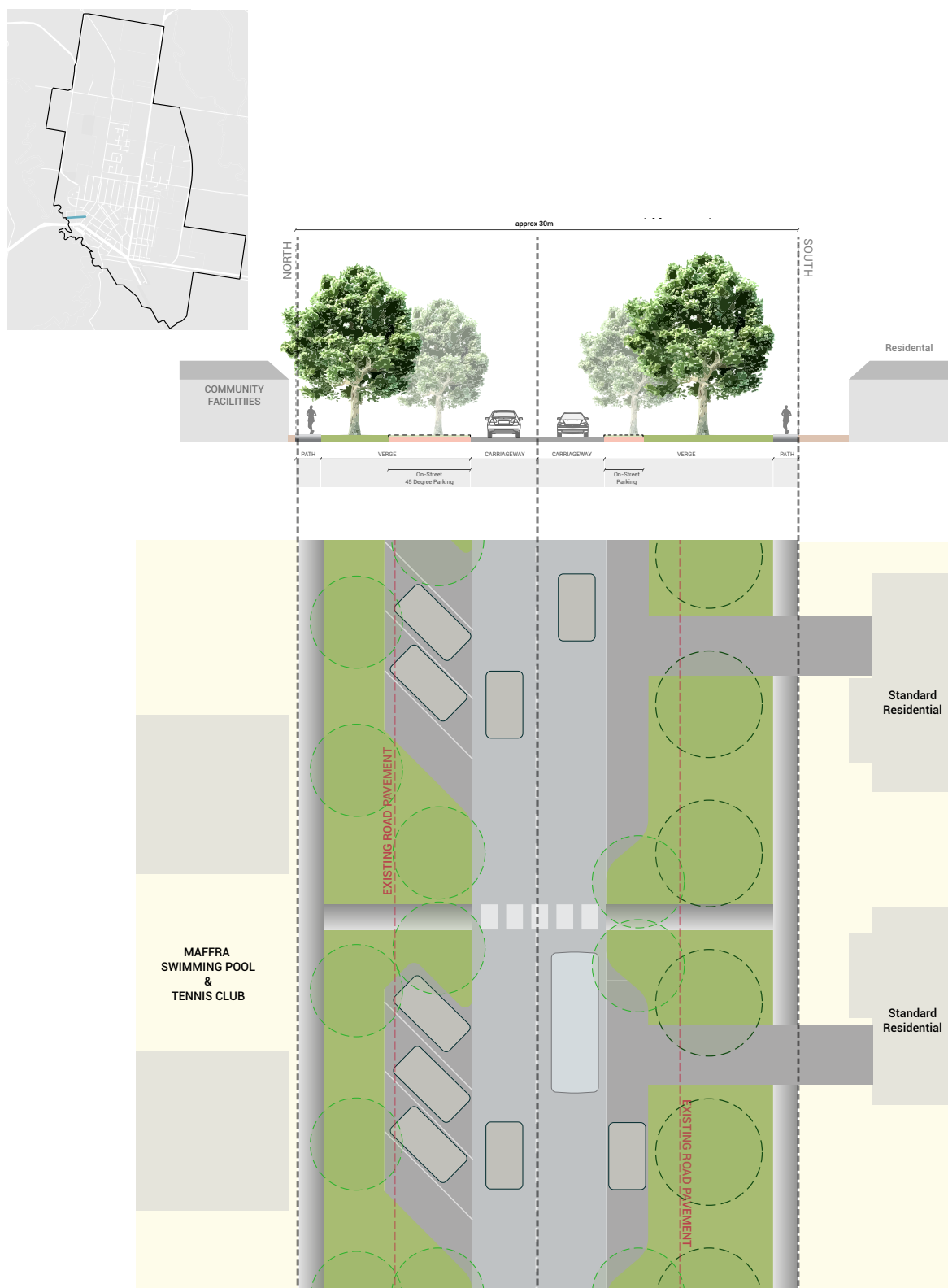
Figure 26: Reduced Pavement Diagram – Duke Street Cross Section – between River St & McMillan St
