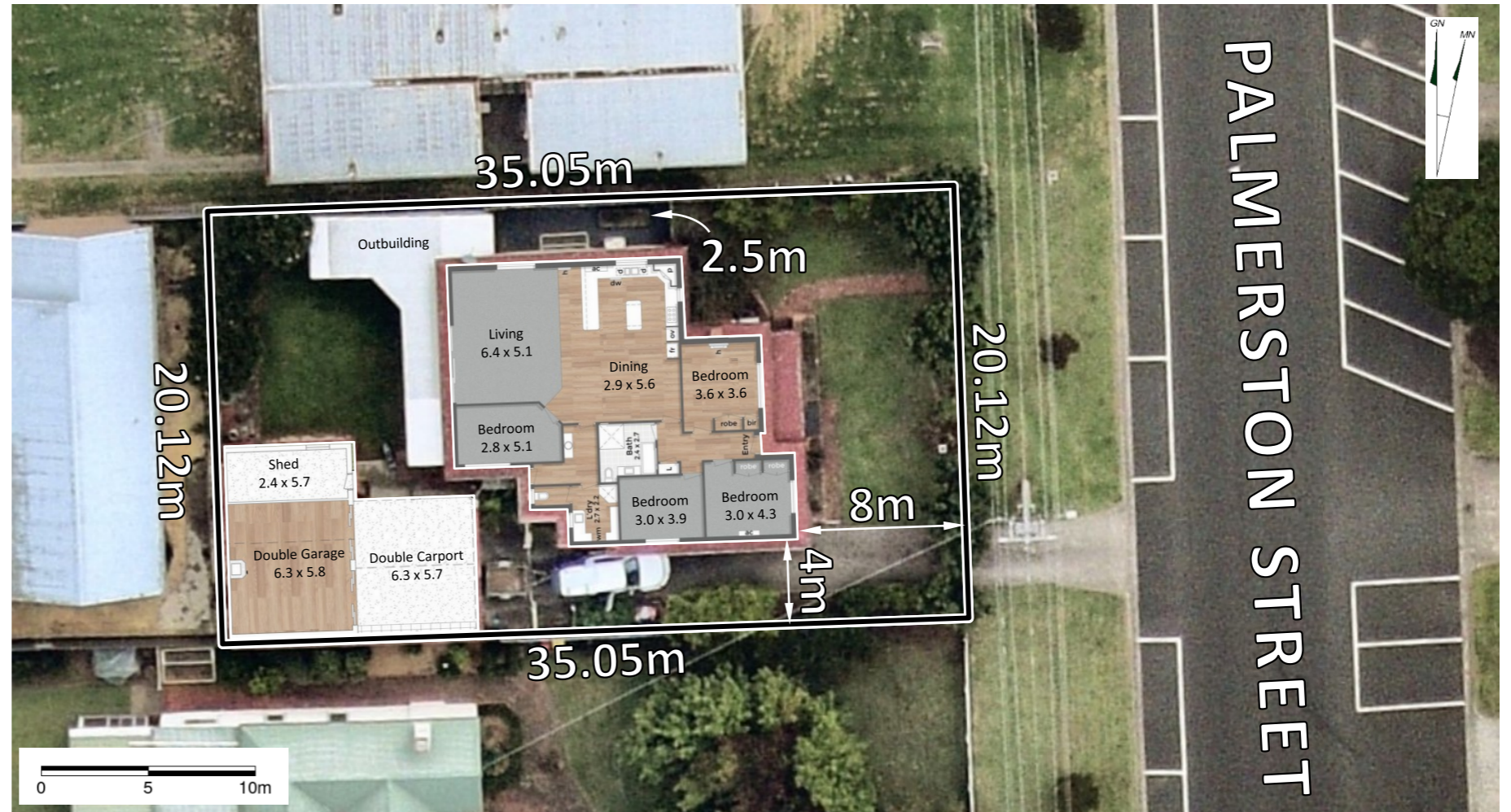
DIMENSIONED AERIAL PHOTO OF THE SUBJECT SITE WITH THE DWELLING FLOOR LAYOUT OVERLAID
