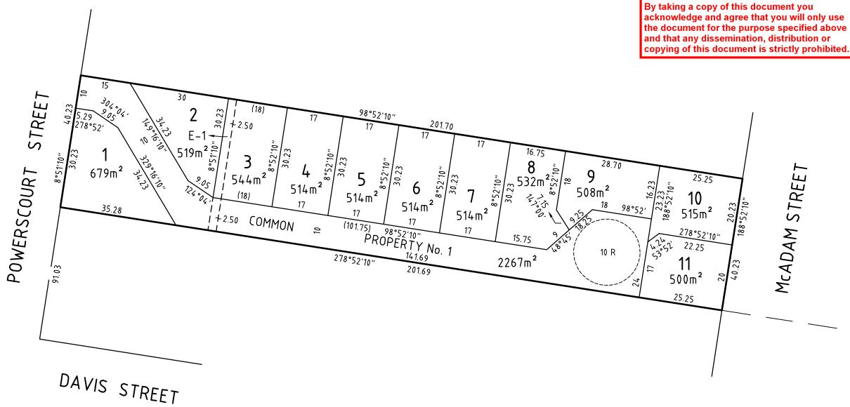
EASEMENT: E-1 PROPOSED EASEMENT FOR PIPELINE OR ANCILLARY PURPOSES OVER EXISTING SEWER MAIN.
