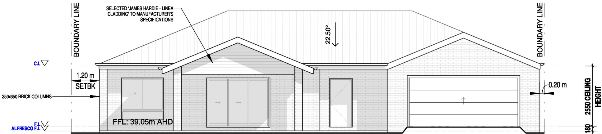
UNIT 2 - WEST ELEVATION 1 : 100
