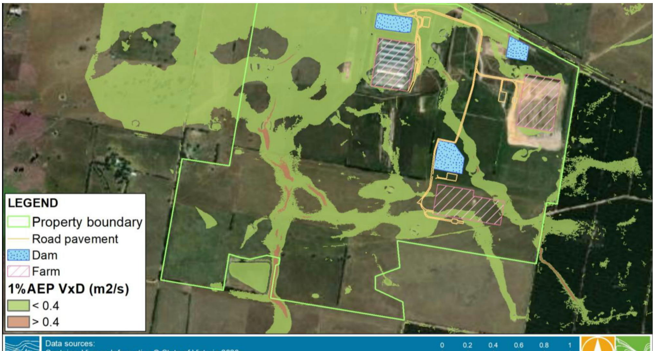
Figure 3-1 1% AEP maximum (V x D) (Existing condition)
