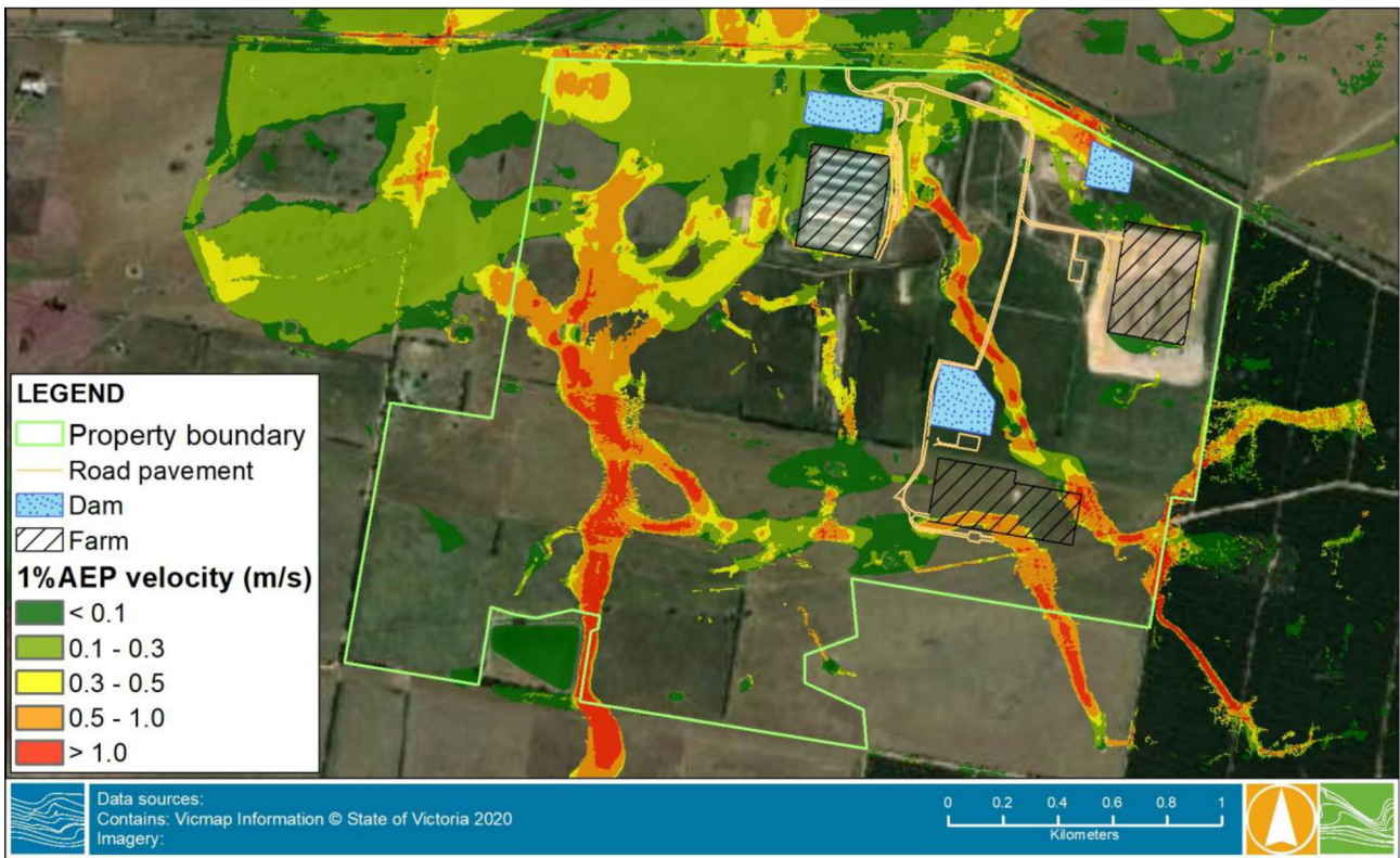
Figure 2-4 1%AEP velocity in existing condition
