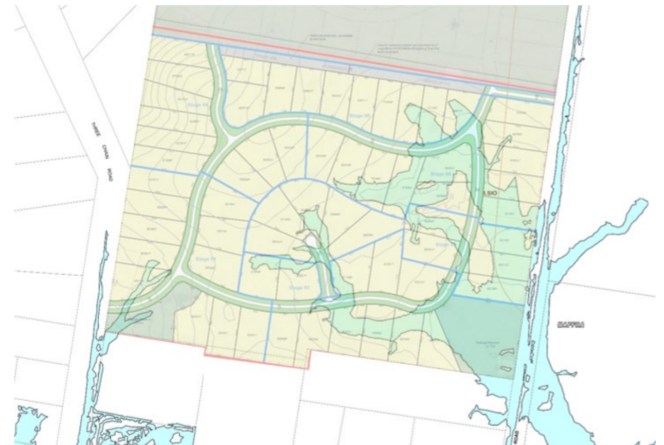
Figure 41: An image of the C125well flood mapping superimposed over the Phase 3 plan
