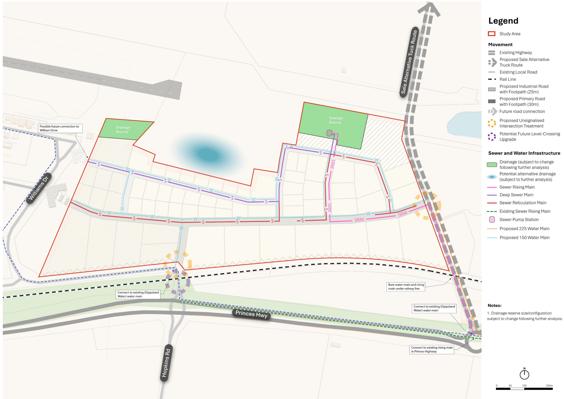
Figure 10. Sewer and Water Plan
