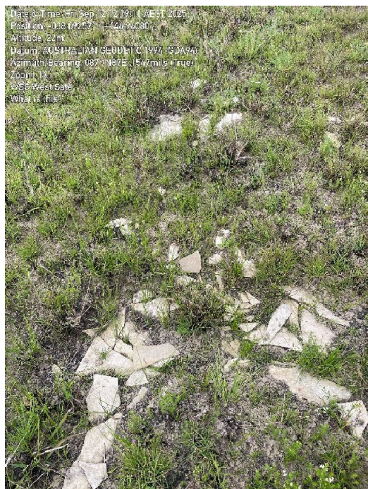
Plate 11. Asbestos in early September
