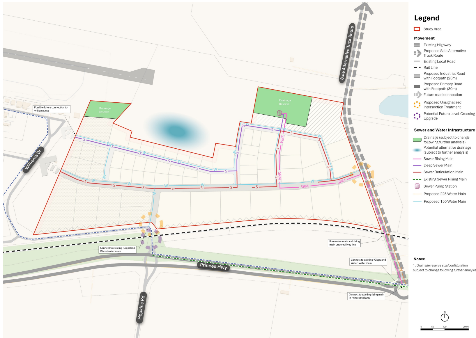
Figure 10. Sewer and Water Plan
