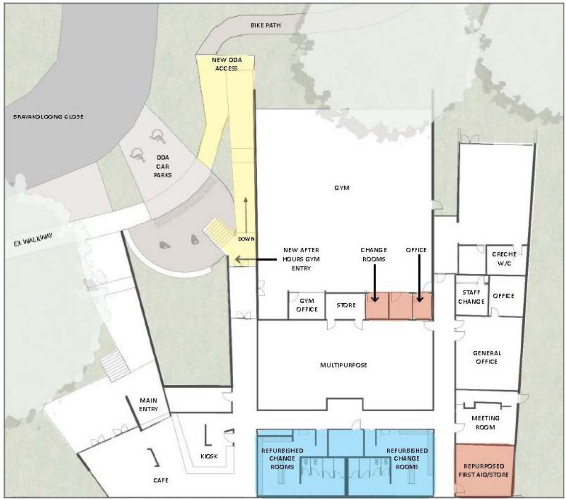
DRY FACILITIES, 24 HOUR ENTRY, CHANGE ROOM & NEW OFFICE
