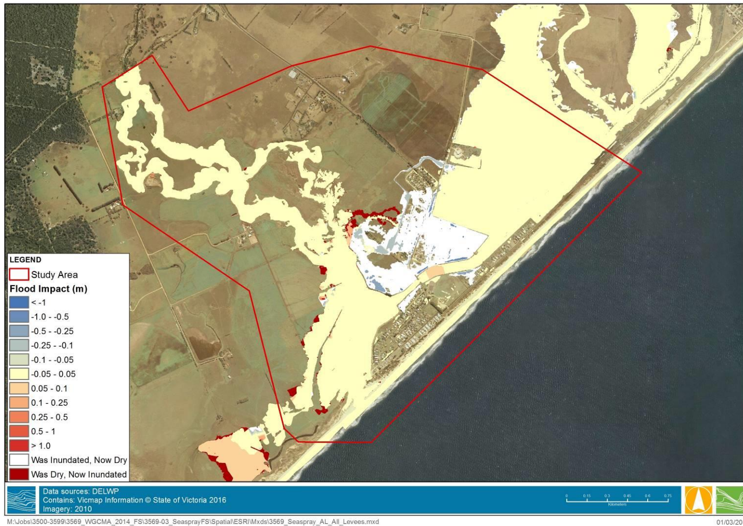
Figure 4-7 Flood Impact of raising all levees about 1% AEP flood level
