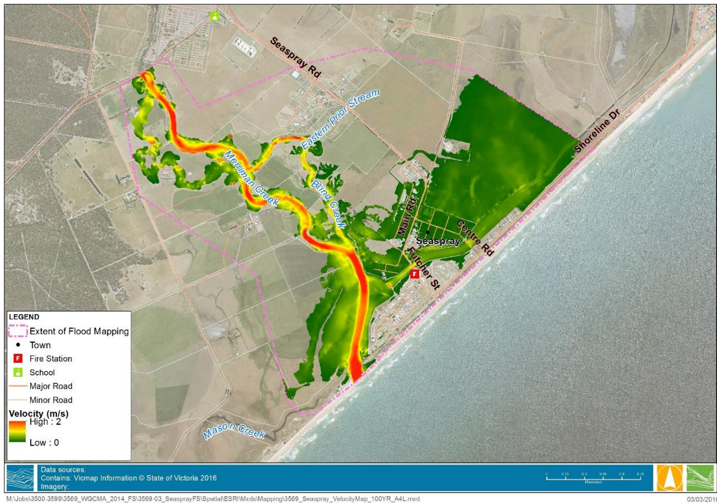
Figure 7-2 Design 1% AEP Peak Flood Velocity Map
