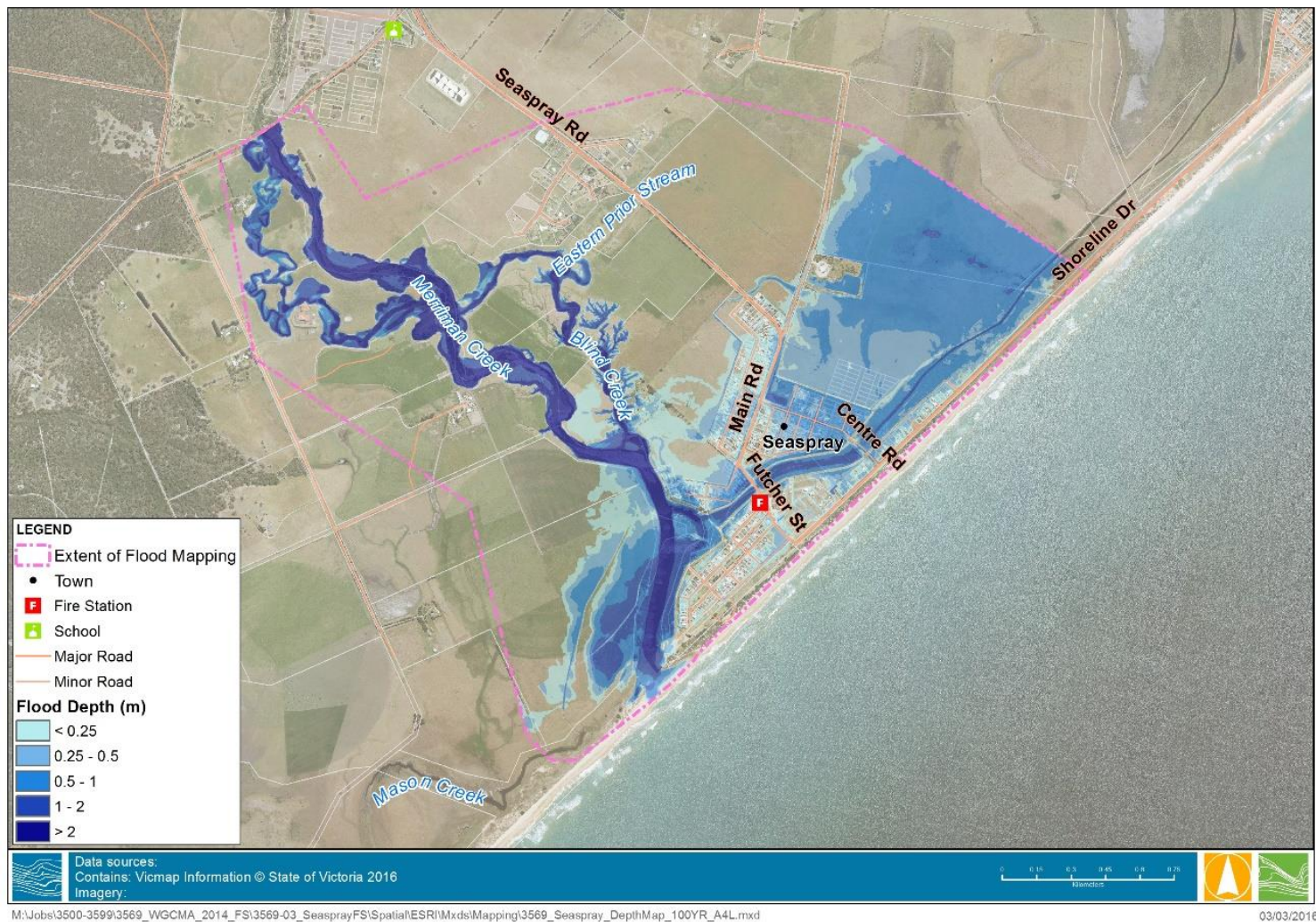
Figure 7-1 Design 1% Flood Depth Map
