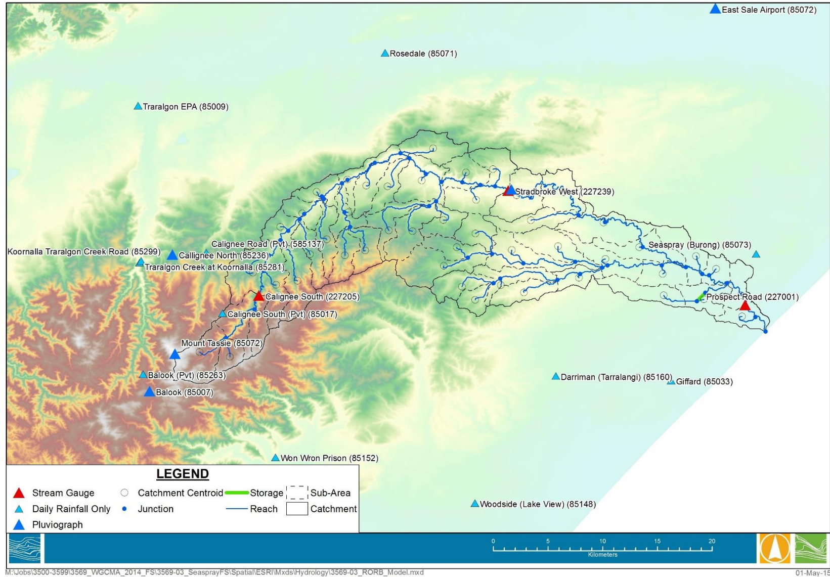
Figure 3-12 RORB model structure
