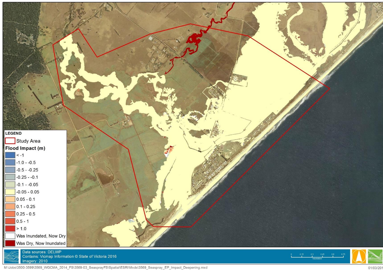
Figure 4-2 Flood Impact of Deepening Easter Prior Stream
