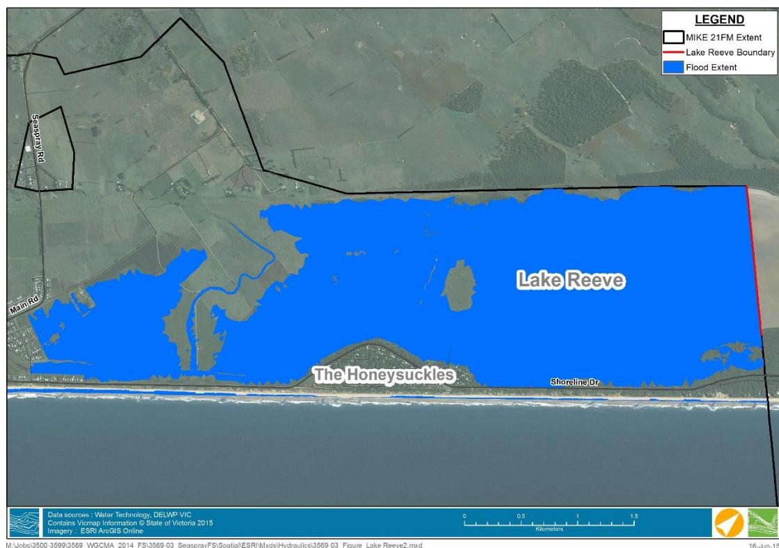
Figure 6-9 Flood Extent with water levels at Lake Reeve raised to 1.37 m AHD
