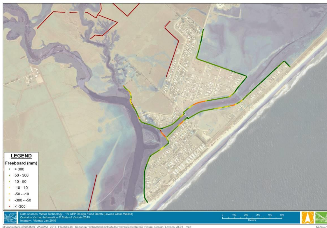
Figure 4-5 Vulnerability of existing levees in the 1% AEP flood event
