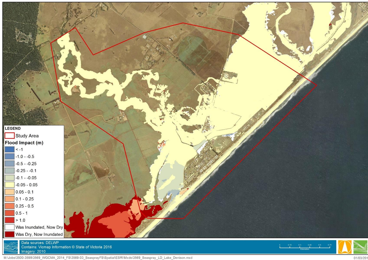
Figure 4-4 Flood Impact of Increased Water Storage in Mason Creek, towards Lake Denison
