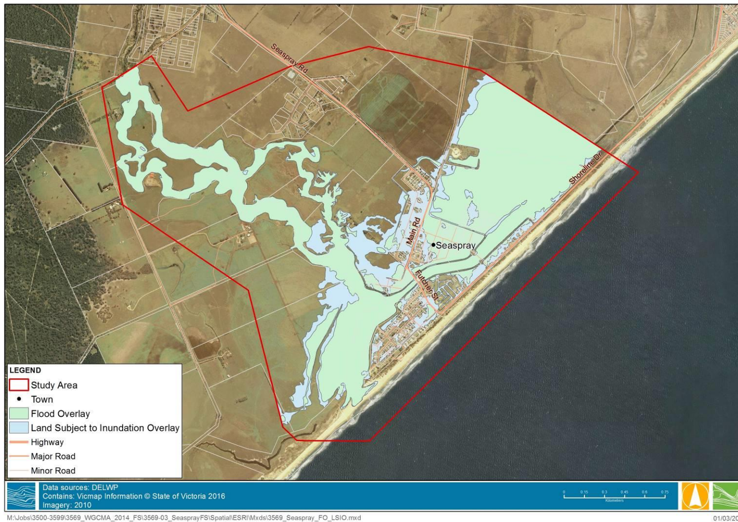
Figure 3-4 Draft LSI0 and FO Map for Existing Conditions
