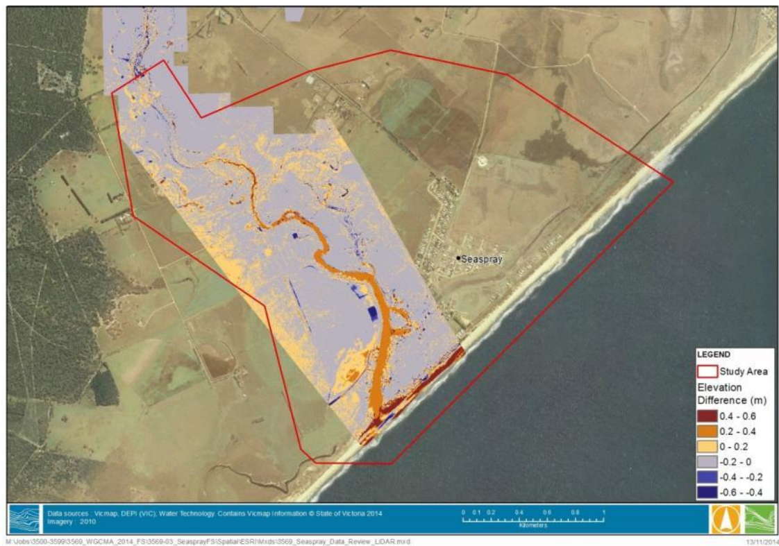
Figure 6-2 LiDAR comparison - Rivers LiDAR DEM minus Coastal DEM
