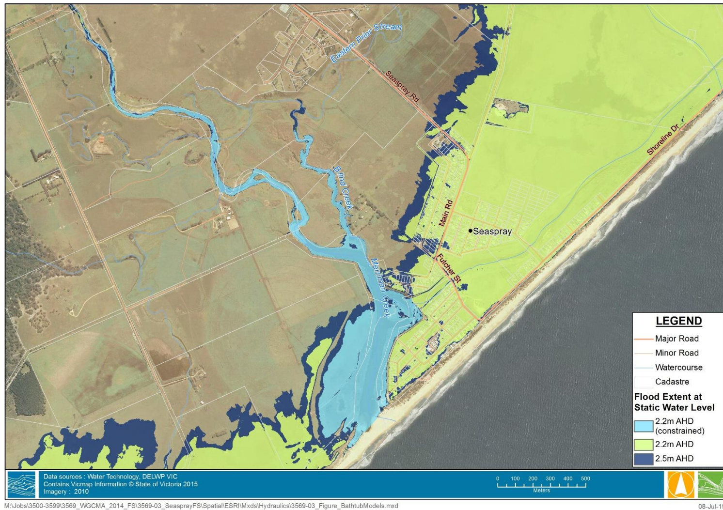
Figure 6-2 Bathtub Inundation Extents at Seaspray for Berm Heights of 2.2 m and 2.5 m AHD
