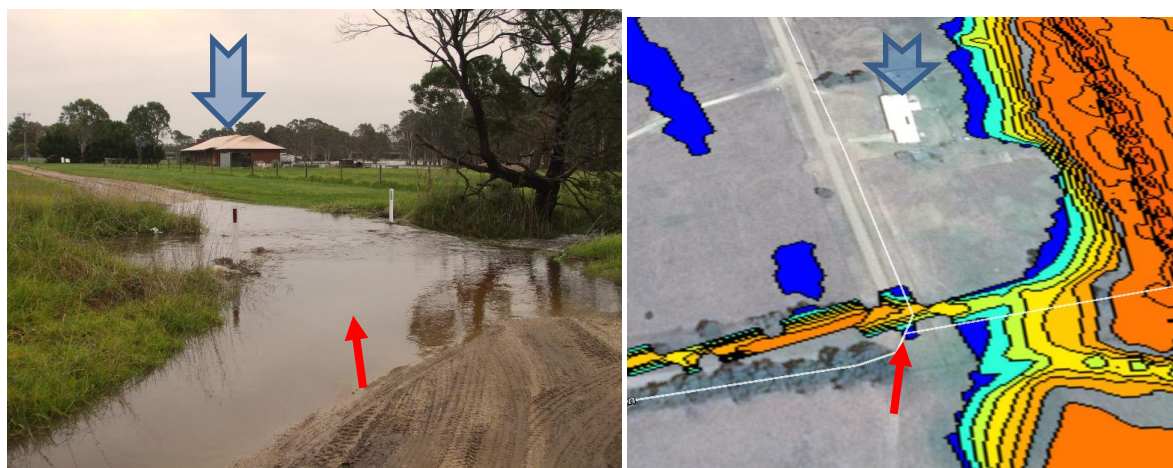
Figure 5-28 June 2012 hydraulic model results compared to photograph from the WSC Rosedale- Mill Lane - 5 th June 2012
