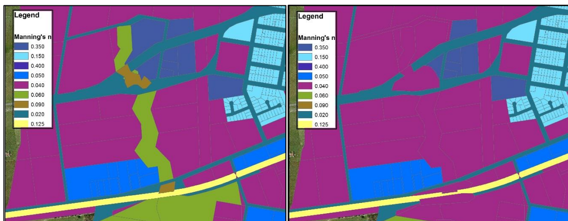
Figure 9-2 Manning’s roughness applied inside the Blind Joes Creek LHS design modelling RHS roughness tested.
