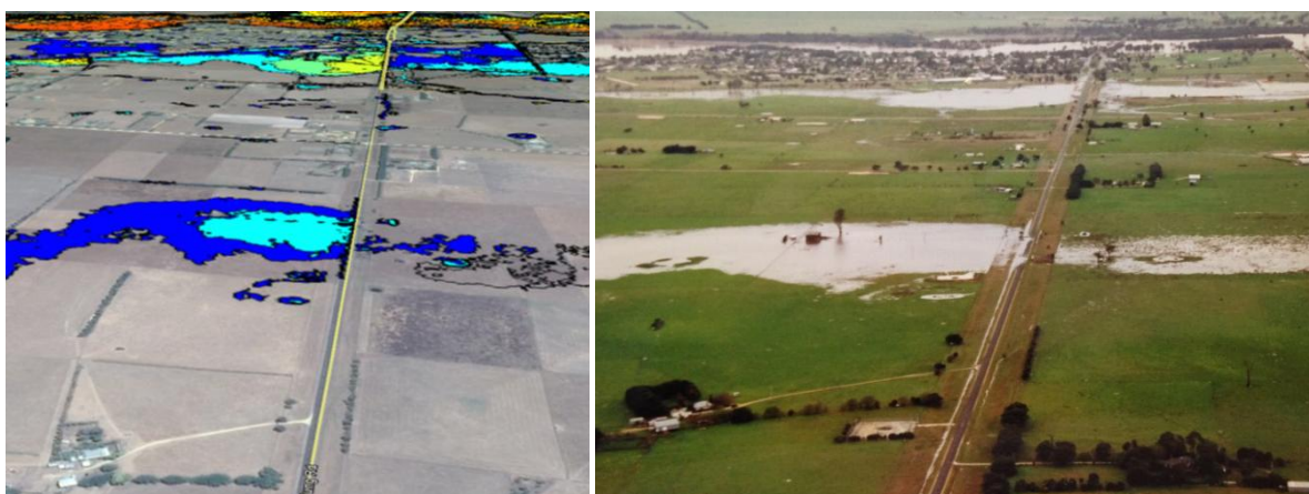
Figure 5-16 September 1993 hydraulic model results compared with oblique aerial photographic record – Willung Road south of town
