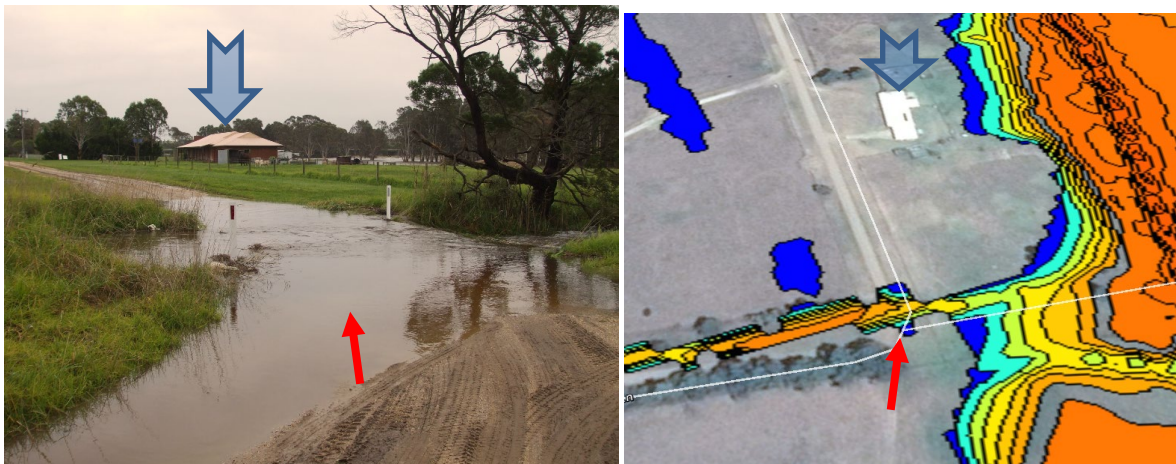
Figure 5-28 June 2012 hydraulic model results compared to photograph from the WSC Rosedale-Mill Lane - 5 th June 2012
