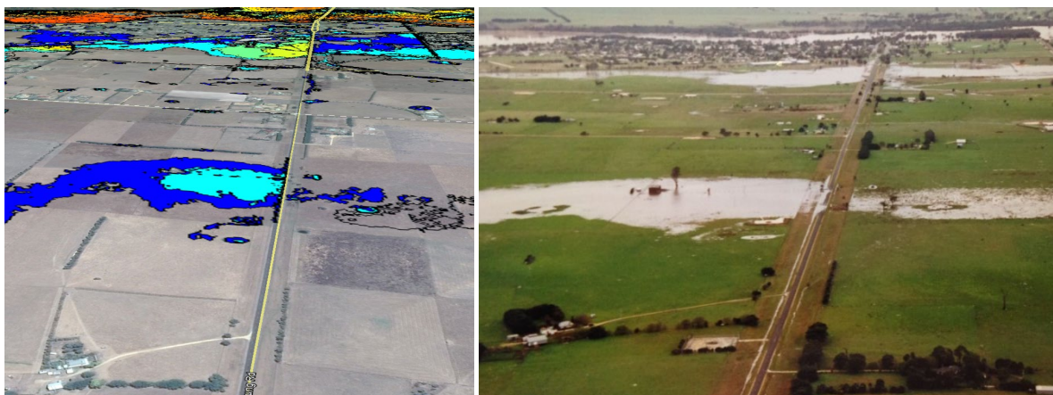
Figure 5-16 September 1993 hydraulic model results compared with oblique aerial photographic record – Willung Road south of town
