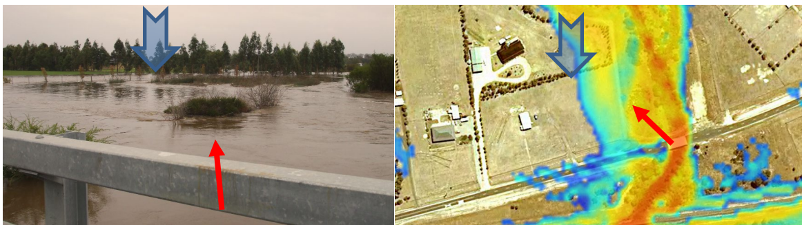
Figure 5-24 June 2012 hydraulic model results compared to photograph from the WSC Rosedale-Cansick Street Bridge - 5 th June 2012
