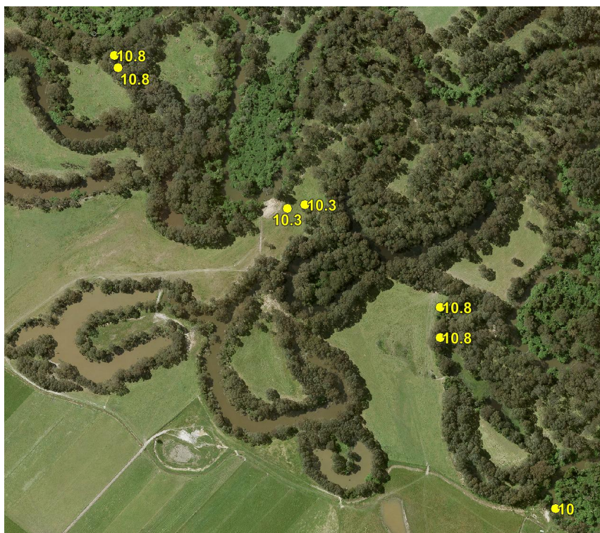
n Figure 10-7 Example of duplicate flood marks indicating potential horizontal error and inconsistent vertical levels of 1978 flood marks
